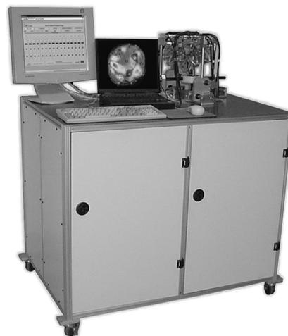
Figure 14: Photograph of the dynamic optical tomographic imager developed in our lab.
