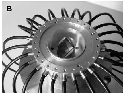
Figure 2: Photograph of the optical D-MUX. A) complete view of the unit (height ~15") with optical fibers attached to it. B) Detailed view of the rotating mirror with the in-coupling optics removed.
